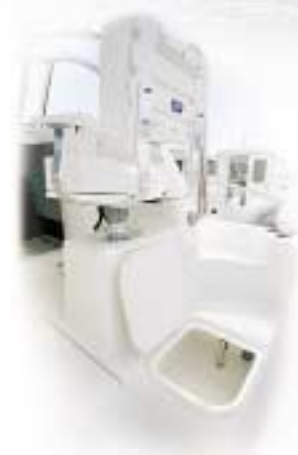
900 Commander & 750 Commander. Like any serious fishing machine, there is a standard bait well with a seawater circulation pump.
