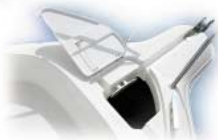
630 Commander. A bow roller, recessed anchor line channel, in-line cleat and anchor locker are professional quality on the 630 series.
